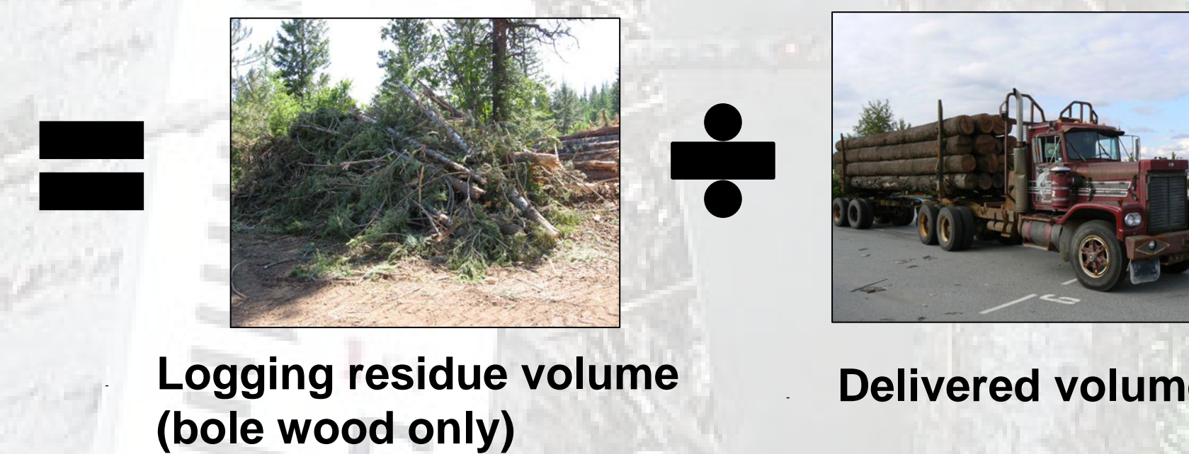
FIGURE 5: The growing stock residue factor, F3- cubic feet of logging residue vs. cubic feet of mill delivered timber
